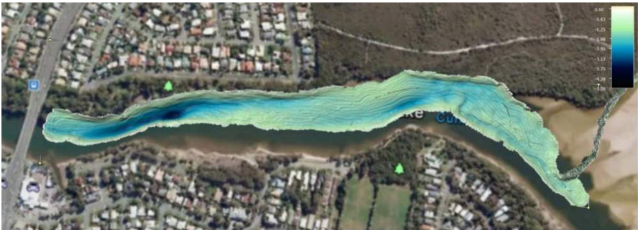
Figure 29: Extract of bathymetry survey from Acoustic Imaging ‘Currimundi Lake Survey’ (December 2015)
