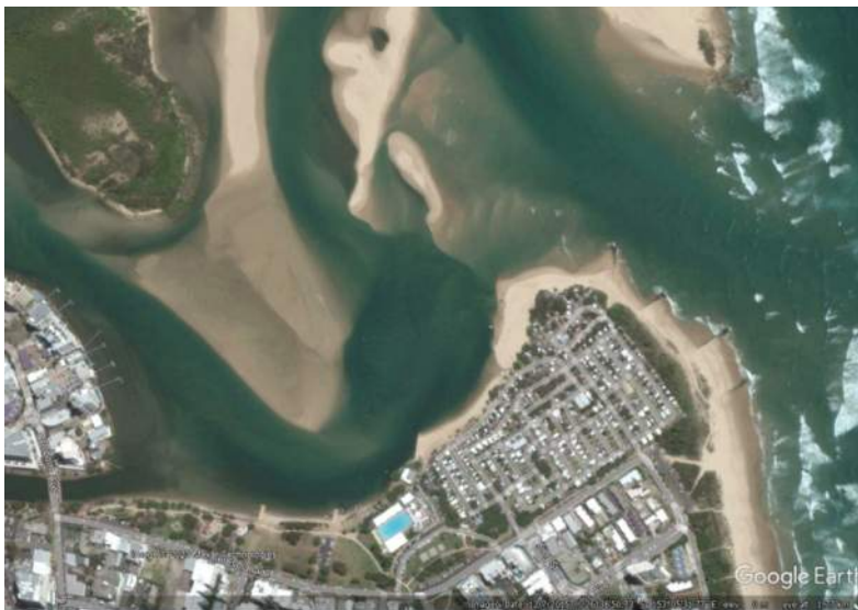
Figure 21: Google Earth aerial image showing minimal sand spit extending from Cotton Tree resulting in relatively exposed conditions at the proposed site
