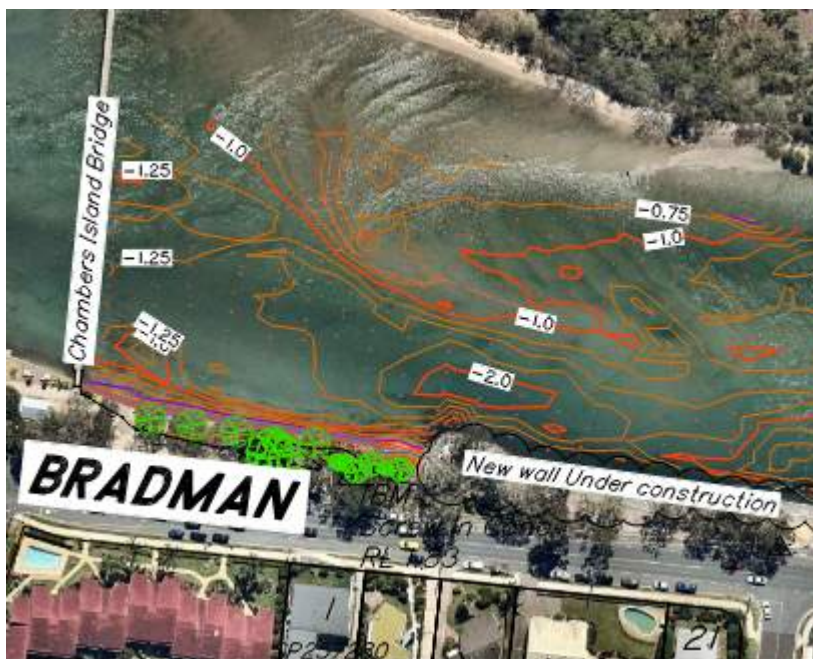
Figure 14: Extract of hydrographic survey by DSQ Land Surveyors (Dated 18.09.18). Note levels are in AHD
