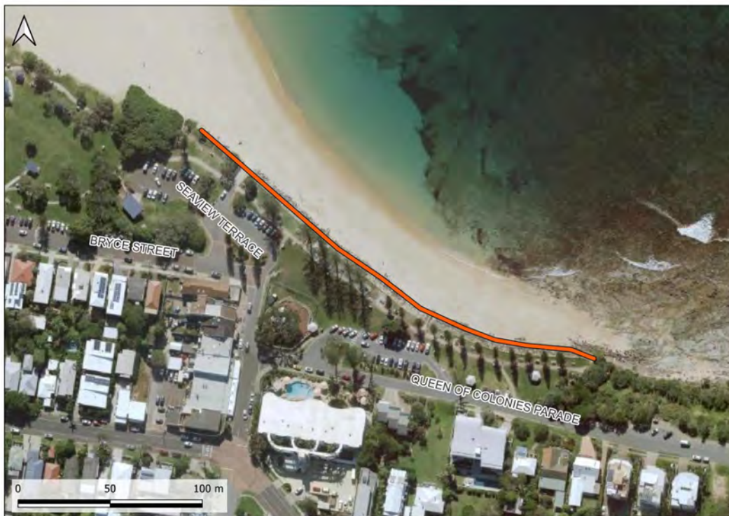
Figure 29-3: Extent of proposed Moffat Beach revetment after expansion (Unit O16, sub-unit A and B)
